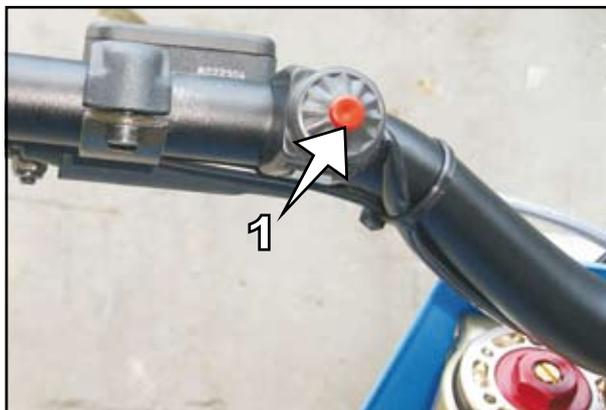
**COMBINATION SWITCH WITH BACKLIT DIGITAL ELECTRONIC SPEEDOMETER (END/SMR/SMM)**
