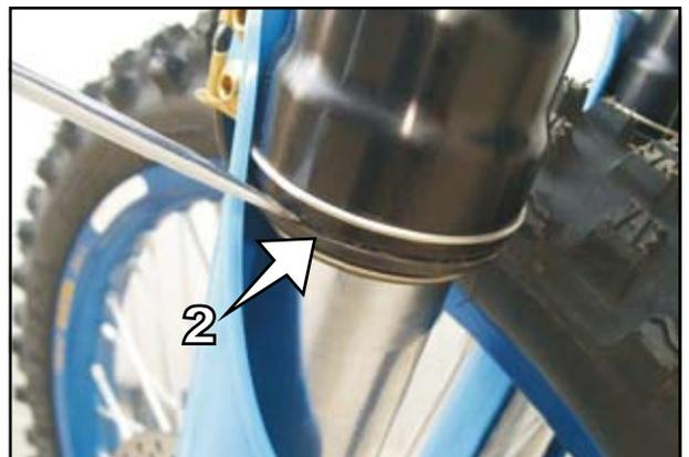
Clean the dust scraper, the outside legs and the rods carefully. Oil them well with silicone spray or with engine oil. Finally, push the dust scraper manually into the outside legs.
