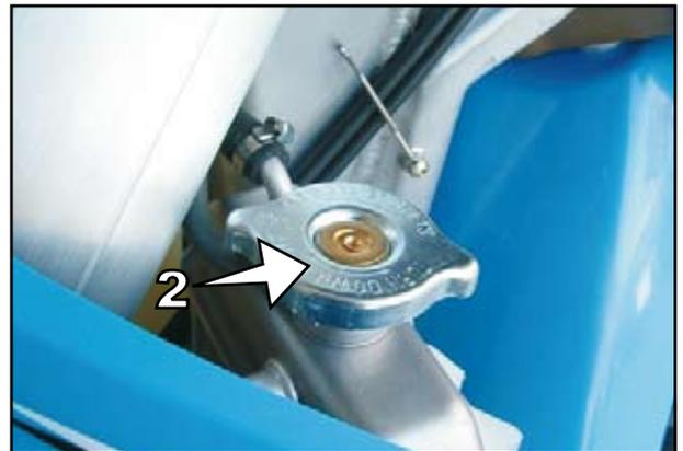
The coolant liquid is a mixture of antifreeze at 40% and water at 60%. The antifreeze protection limit must however be at least -25°C.
